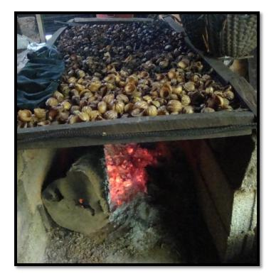
Figure 3: Traditional open fire method to dry the Uppage fruit (requires nearly 22 kilograms of fuel wood to obtain one kilogram of Uppage dry rind). As we have installed such driers in the places where availability of *Garcinia gummigutta* is more and these driers could be of significant use to them. Further, the area is situated within thick forest range and containing enumerable forest species, reduction in deforestation by participatory method would be the positive outcome.
